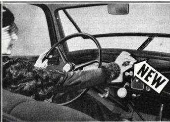
**NEW DODGE "7-POINT VENTILATION"**—An improved and perfected ventilating system. (1) Cowl ventilator. (2) Windshield opens or closes by means of crank on the instrument board. (3) Front half of forward window may be swung open in "butterfly" fashion. (4) Rear half of the window can be raised or lowered independently of the "butterfly". (5) Both halves of the forward window may be locked into a single unit and raised or lowered together, just as with a regular window. (6) Rear door window,
